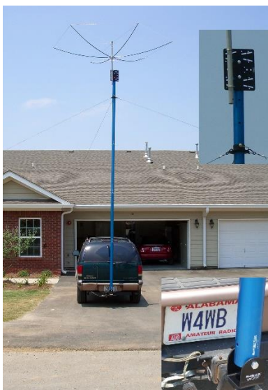
Figure 8. Hex-Beam for 15 m assembled from the Hex-Pac mounted on a Blue Sky Lite mast.
